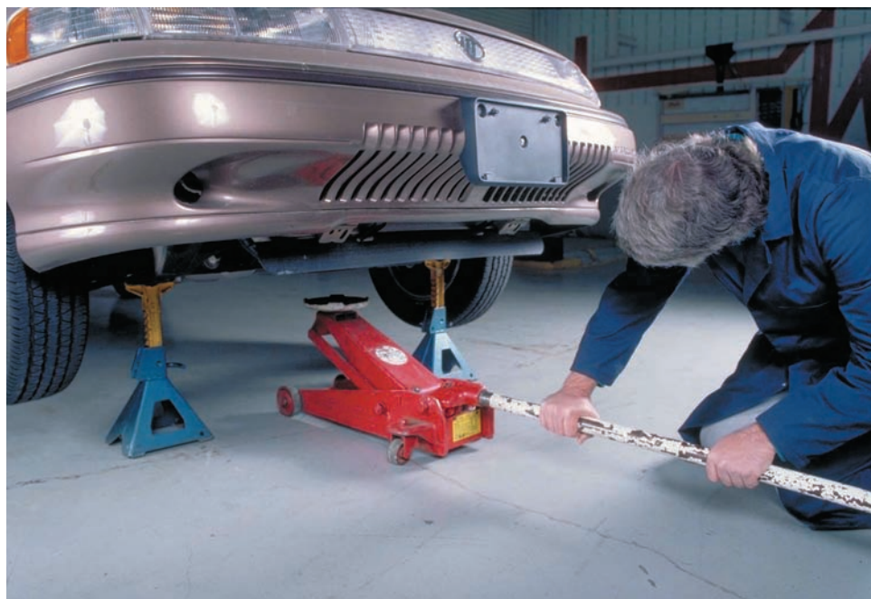
Figure 1-2 Support a vehicle on safety stands such as these and move the jack out of the way.
