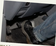
P10-4 To test the operation of the vacuum check valve, shut off the engine and wait for 5 minutes. Apply the brakes. There should be power assist on at least one pedal stroke. If power assist is not present, check for application.
