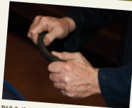
P10-3 If you do not feel a strong vacuum in step 2, shut off the engine. Remove the hose, and see if it is collapsed, crimped, or clogged. Replace it if needed.
