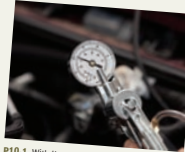
P10-1 With the engine idling, attach a vacuum gauge to an intake manifold port. Any reading below 14 in. Hg of vacuum may indicate an engine problem.
