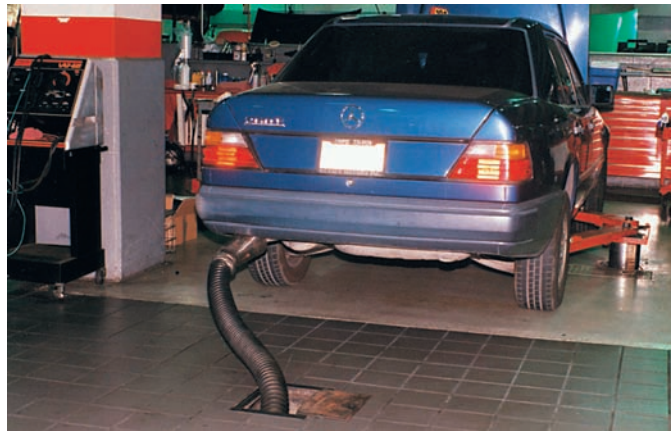
Figure 1-4 When running an engine in a shop, always connect the exhaust to the ventilation system.
