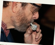
P10-6 Test the check valve by blowing into the intake manifold end of the valve. There should be a complete blockage of airflow.
